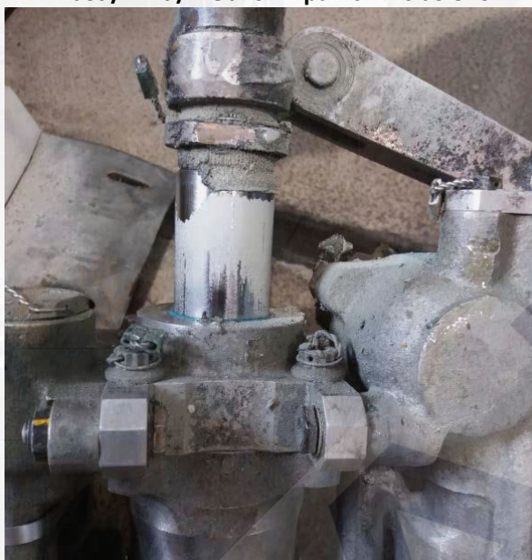
Dust / Dirt / Debris in paint - Inclusions
