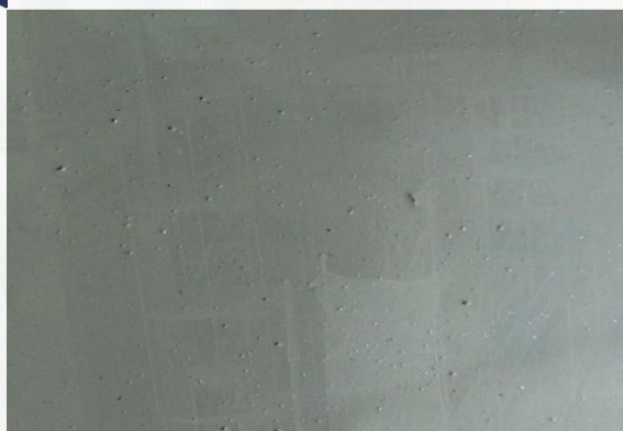
Dust / Dirt / Debris in paint - Inclusions
