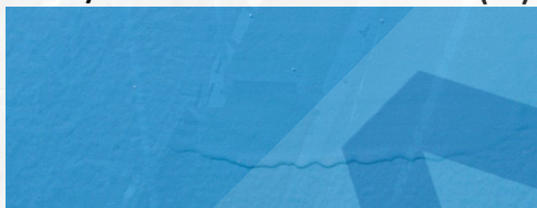
Runs / Sags (Note around doors / cut outs and panel edges, trailing edges etc)
